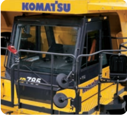
ROPS/FOPS to ISO 3471 ROPS and ISO 3449 FOPS Level II standard
