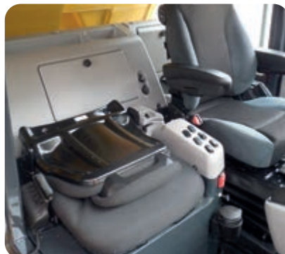
The full size trainer seat is foldable and has a 2-point retractable seat belt
