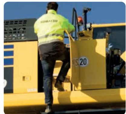
Handrails and anti-slip plates
