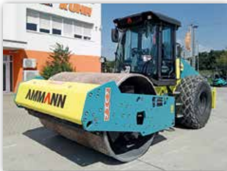
Ammann roller ARS150 upgraded with ACE Force Compaction Measuring (digitised sealing reports for the construction sites)
